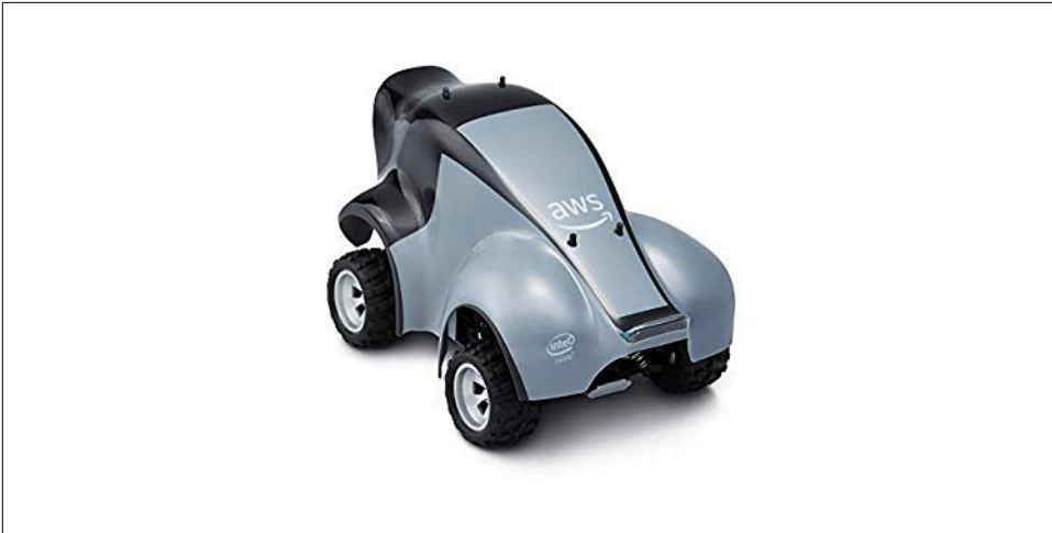
Figure 17-1. The AWS DeepRacer one-eighth-scale autonomous car
