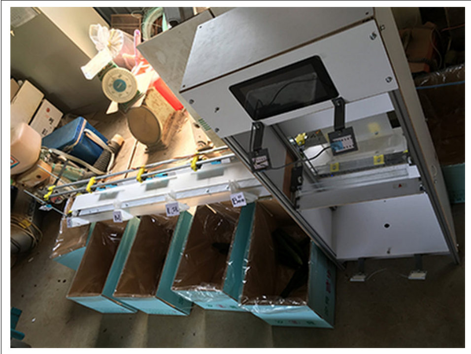
Figure 15-14. Makoto Koike's cucumber sorting machine ( image source )
