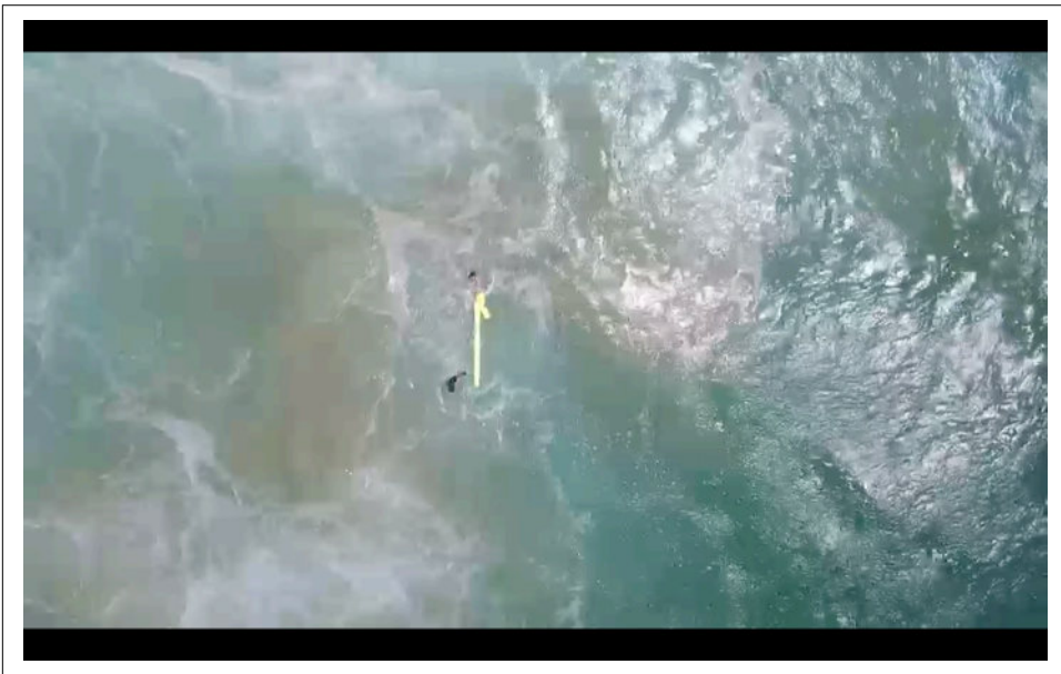
Figure 8-26. Drone identifies two stranded swimmers and releases an inflatable pod that they cling onto ( image source )
